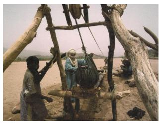
This photograph shows how a pulley system in Niger, Africa is used to get water from a well. A wooden structure was built to support a pulley. One end of a rope is passed over the pulley and attached to an animal-hide bucket. By attaching the other end of the rope to a donkey, the bucket can be raised and lowered. This piece of equipment doesn't work by itself. Someone or something has to pull the
