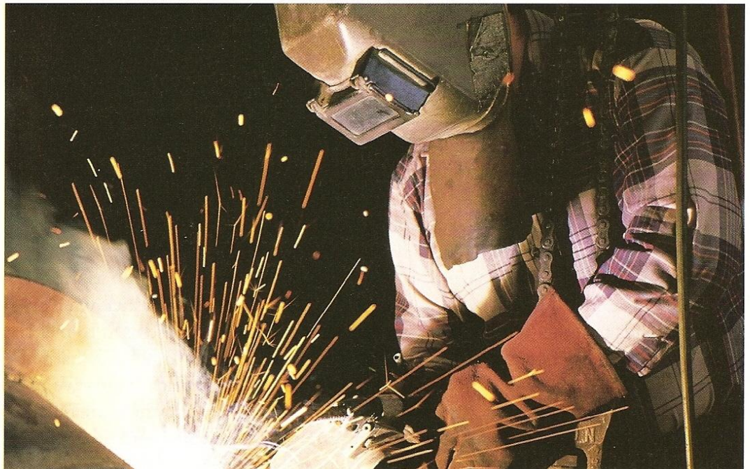
Figure 13.23 Welders use a dark mask to protect their eyes and to see white-hot joints clearly.
